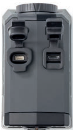
Micro HDMI and Micro USB ports
